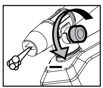
**Reduce Detergent Used**Turn adjuster anti-clockwise to reduce the amount of detergent mixture used.
