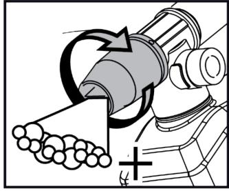
**Wide Water Jet**Rotate nozzle clockwise to create a wide spread water jet.
