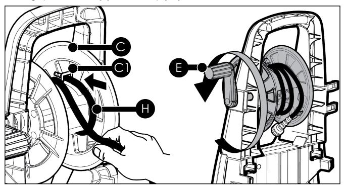
8. When winding the hose storage reel, make sure it is tidy and not overlapping at all.
