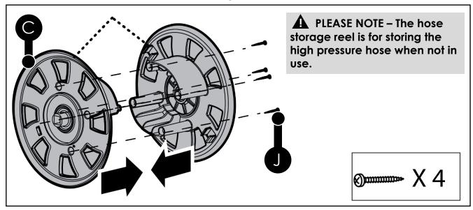
2. Push the hose storage reel (C) into place on the carry handle (B).
