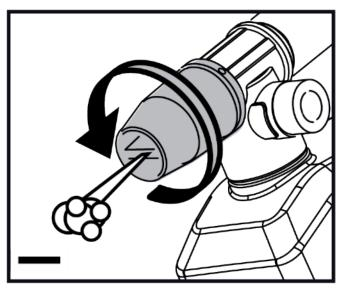
Narrow Water Jet Rotate nozzle anti-clockwise to create a narrow water jet.
